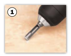
The drill needs to run before hitting the surface. To avoid the sliding of the drill, start with an angle of 45°.
